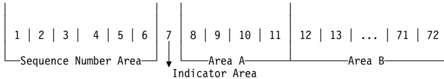
Figure 1. Reference Format for COBOL Source Line
